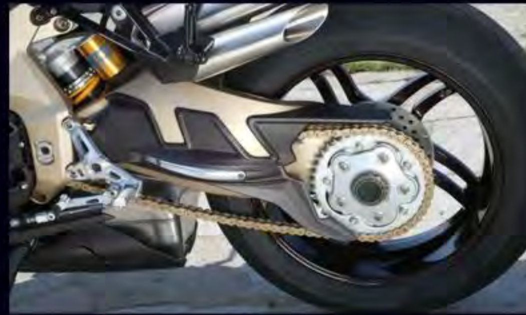
(Above) The single-sided swingarm carried in an adjustable pivot is a direct carry-over from the previous model. (Right) The dash is substantially improved compared to MV's of old.
