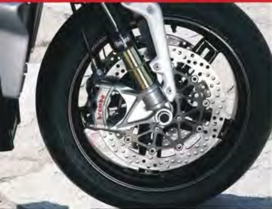
(Above) Brembo has fitted their latest Stylema calipers in the same fashion as the Ducati Panigale V4 R and the Aprilia RSV4 1100 Factory. (Below) Isn't that one of the most stunning back-ends you've ever seen?
