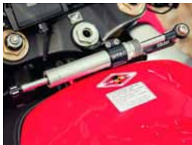
Sprint steering damper is a sensible mod
